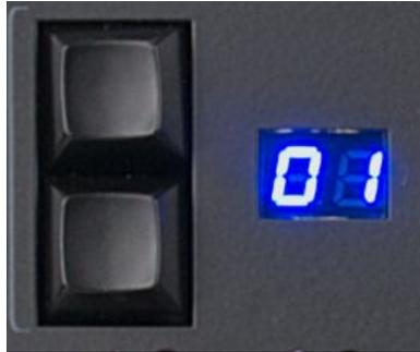
There are 2 separate sets of page control buttons, one for the Playback Faders and another for the Matrix buttons. Paging essentially gives you additional virtual sets of faders and matrix buttons to work with. Paging can be controlled by your lighting software or by the **MIDICON-2™** controller via MIDI channel paging. If your software can control the paging you can have up to 99 pages to work with.
