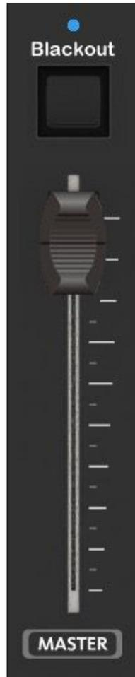
The master fader is generally used to control the overall level of the stage lights but can also be used to control other things like speed or be used as another playback fader. This fader is not tied to the page controls.
