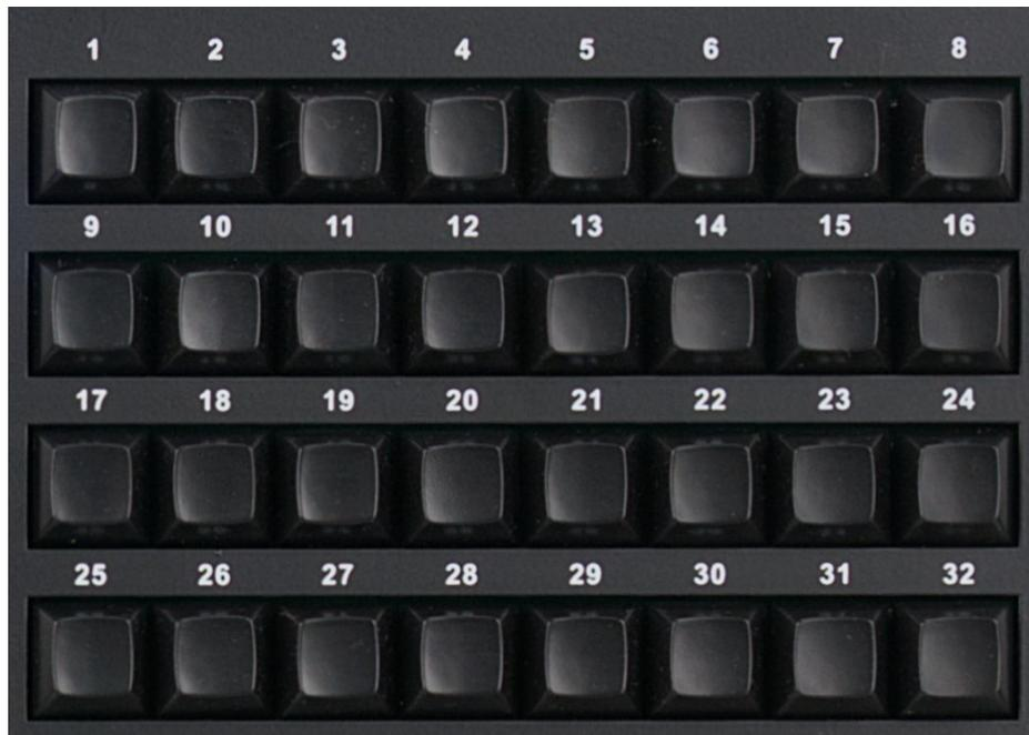
These 32 buttons can be used to call lighting effects, scenes, colors, etc. If your lighting software does not support the **MIDICON-2™** as plug and play, you will have to link each button to a function using the setup menu in your software. Refer to your software manual for instructions, as this will be different for each program.
