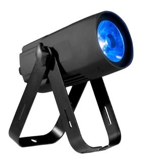
The Saber Spot RGBW is a compact Pinspot with smooth RGBW color mixing from one 15W 4-in-1 Quad LED, and features DMX-512, flicker-free operation, 64 built-in color macros, strobing, electronic dimming and has a 4-Button DMX display system on the rear panel. Its built-in ACL lens produces a razor sharp 4-degree beam angle. Included are 2 additional fresnel lenses of 10 & 45 degree
