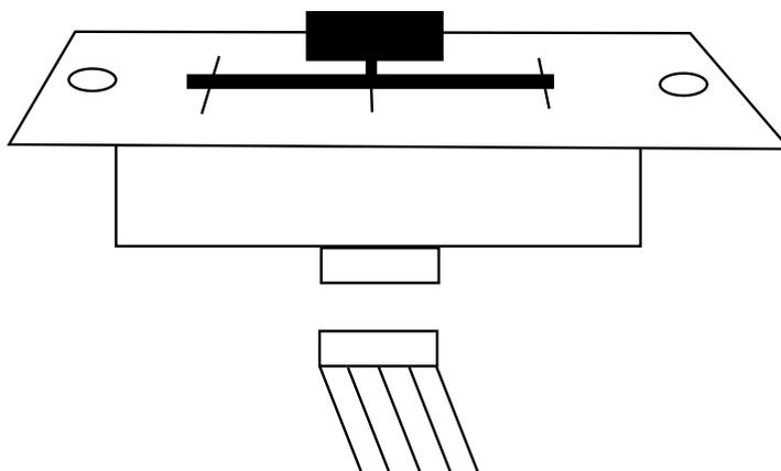
The crossfader is “Hot Changeable” which means it may be replaced at any time, even when power is applied. Only replace with American Audio Feather Fader Plus. Replacing with any other model fader may seriously damage your mixer.
