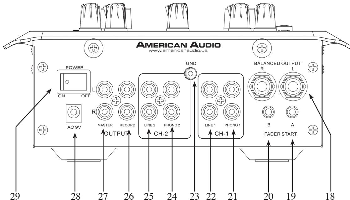
**18. BALANCED 1/4" MASTER OUTPUT JACKS** - The Master Output includes a pair of 1/4" Balanced jacks as well as a pair of *RCA UNBALANCED JACKS* (27). The 3-pin XLR jacks send a high current balanced output signal. These jacks should be used when you will be driving an amp or other audio equipment with a balanced input, or whenever you will be running a signal line greater than 15 feet. Always, use these jacks whenever possible.
