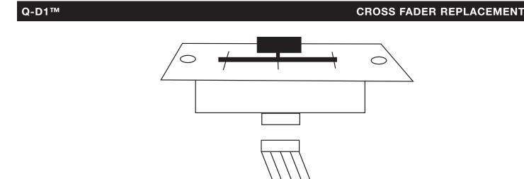
The crossfader is "Hot Changeable" which means it may be replaced at any time, even when power is applied. Only replace with American Audio Feather Fader Plus. Replacing with any other model fader may seriously damage your mixer.
