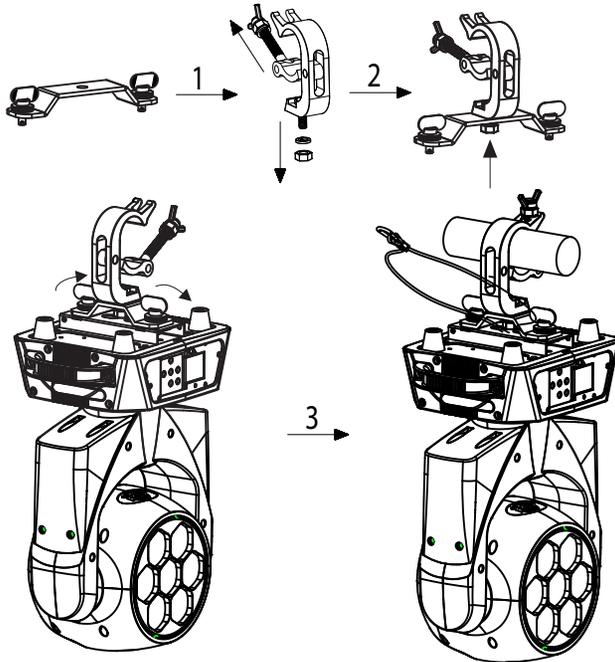
Screw one clamp each via a M12 screw and nut onto the Omega holders. Insert the quick-lock fasteners of the Omega holders into the respective holes on the bottom of the Vizi Hex Wash7. Tighten the quick-lock fasteners fully clockwise. Install the second Omega holder. Pull the safety-cable through the holes on the bottom of the base and over the trussing system or a safe fixation spot. Insert the end in the carabine and tighten the safety screw.
