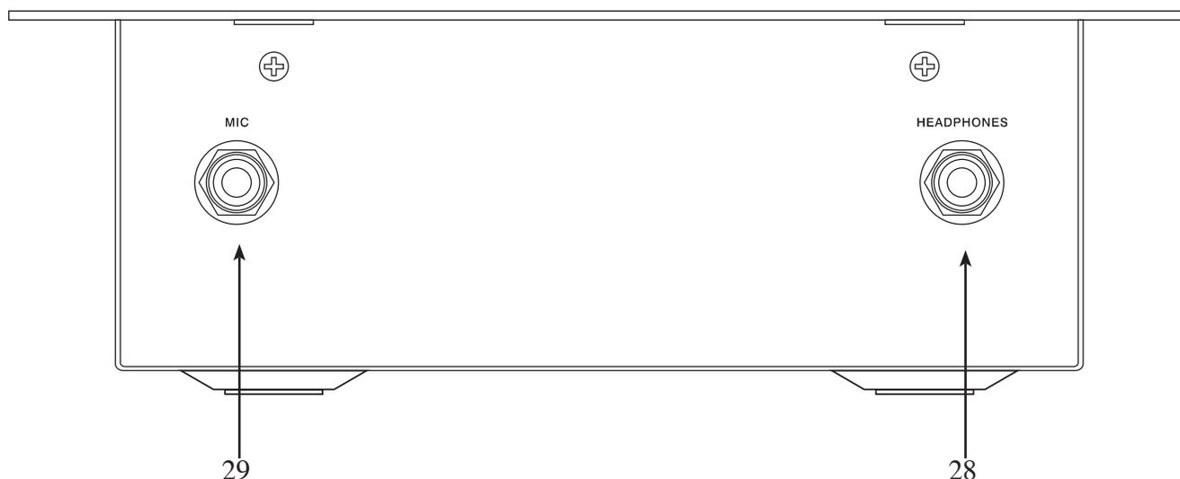
**28. HEADPHONE OUTPUT JACK** - This jack is used to connect your headphones to the mixer allowing you to monitor the cue source. Use headphones only rated at 8 ohms to 32 ohms. Most DJ headphones are rated at 16 ohm, these are highly recommended. Always be sure the *CUE LEVEL VOLUME (5)* is set to minimum before you put the headphones on.
