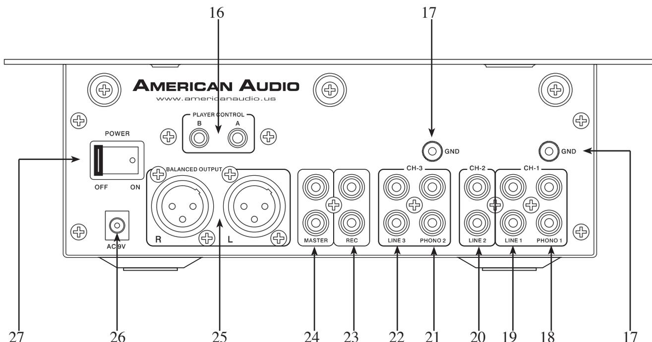
**16. PLAYER CONTROL** - These jacks are used to control the “Q-Start” function between the mixer and a compatible American Audio CD Player. Input mini plugs from CD player controller into these jacks, input CD 1 into jack A and CD 2 into jack B.
