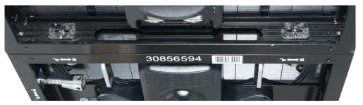
2. Push locking vertical connectors up through their corresponding slotted vertical tab-keyed connector sockets
