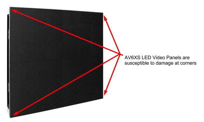
Because these are ESD sensitive units, use ESD precautions when removing the AV6XS LED Video Panels from their flight case (ESD gloves, protective clothing, wrist straps, etc.). In addition to using standard ESD precautions, to reduce static building friction, take care to lift the panels without rubbing the LED panel surface along the foam-covered slots, which can generate static electricity that can damage LEDs on AV6XS Panel.
