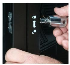
1. Align the locking-tab with tab-keyed connector socket
