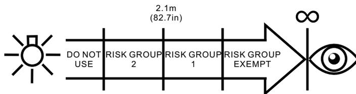
The luminaire should be positioned so that prolonged staring into the luminaire at a distance closer than 2.1 m is not expected.
