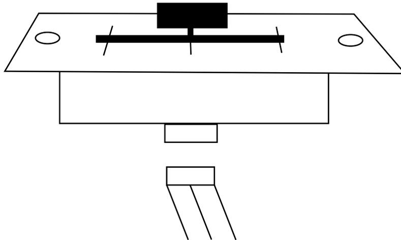
The crossfader is “Hot Swapable” which means it may be replaced at any time, even when power is applied. Only replace with American Audio Part Feather Fader Plus. Replacing with any other model fader may seriously damage your mixer. Please, always use insulated tools.
