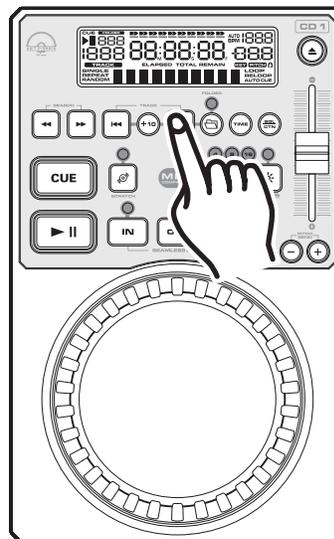
Figure 10: Tapping the forward track button will skip forward to the next track.
