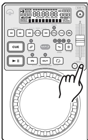
Holding down or tapping on the (+) *PITCH BEND BUTTON* (8) will provide a speed bump in the playback pitch.
