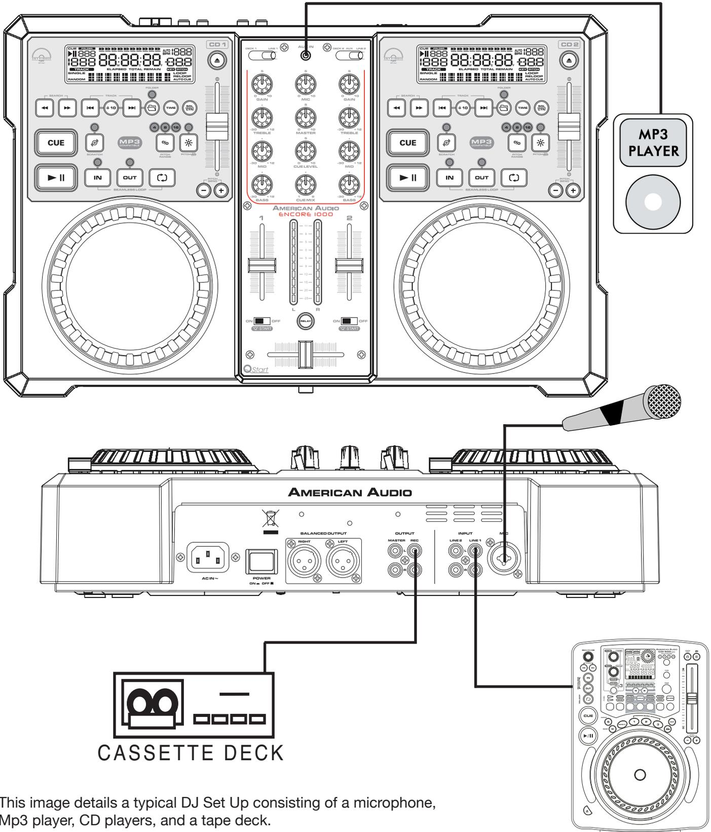
This image details a typical DJ Set Up consisting of a microphone, Mp3 player, CD players, and a tape deck.
