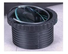
Flip the focus barrel over and insert the new lens. Very carefully insert the retainer ring. Make sure retainer ring is in correctly, flush against the lens. Finally, screw the focus barrel back into the fixture.
