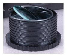
The image to the left illustrates how the focus barrel should look after the lens has been popped out. Remove the lens and retainer ring.
