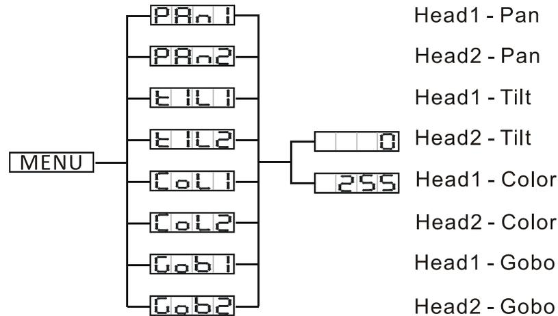
To enter the home position adjustment menu, press the ENTER button for at least 5 seconds. In this submenu you are able to adjust the original position of the pan position, tilt position, color wheel position, and gobo wheel position. When looking at the fixture, with the LED display in front of you, the Master is the moving head on the right, the Slave is the left moving head.
