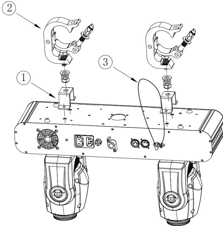
**Attaching Brackets, Clamps, & Safety-Cable:** Screw one clamp via a M12 screw and nut to the included bracket. Attach the bracket using the included screws to the bottom of the Inno Pocket Spot Twins. Attach the eyehole screw to the side of the base and pull the safety-cable through the screw and over the trussing system or a safe fixation spot. Insert the end in the carabine and tighten the safety screw.
