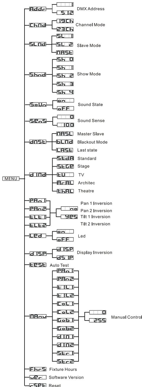
**System Menu:** When making adjustments press **ENTER** to confirm your setup then press and hold the **MENU** button for at least 3 seconds. To exit without making any adjustments press the **MENU** button. The display will lock after 30 seconds, press the **MENU** button for 3 seconds to unlock.
