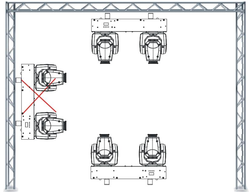
The Inno Pocket Spot Twins is fully operational in two different mounting positions, hanging upside-down from a ceiling or set on a flat level surface. To avoid internal damage to the unit, never mount the unit on its side as illustrated above. Be sure this fixture is kept at least 0.5m away from any flammable materials (decoration etc.). Always use and install the supplied safety cable as a safety measure to prevent accidental damage and/or injury in the event the clamp fails (see next page).
