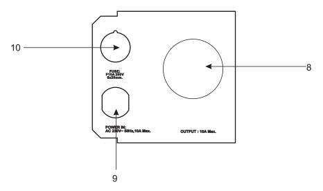
8. Output: One Schuko socket for Output, 10A MAX.
