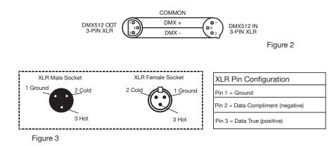
**Special Note: Line Termination.** When longer runs of cable are used, you may need to use a terminator on the last unit to avoid erratic behavior. A terminator is a 110-120 ohm 1/4 watt resistor which is connected between pins 2 and 3 of a male XLR connector (DATA + and DATA -). This unit is inserted in the female XLR connector of the last unit in your daisy chain to terminate the line. Using a cable terminator (ADJ part number Z-DMX/T) will decrease the possibilities of erratic behavior.
