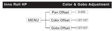
To enter the offset adjustment submenu, press the ENTER button for at least 5 seconds. In this submenu you are able to adjust the original position of the pan, gobo wheel, and color wheel.
