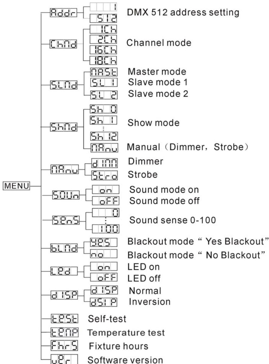
**ADDR - DMX Address Setting via control board -**
