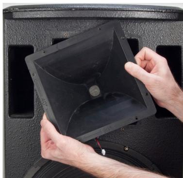
5. After unscrewing and removing the screws, carefully and gently pull the horn out of the housing (not all the way) and rotate the horn 90 degrees.
