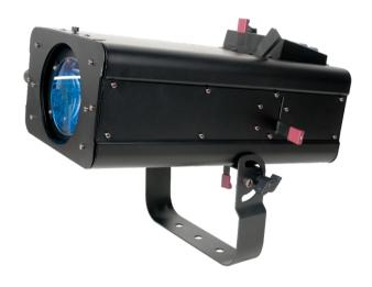
The ADJ FS600LED is a modern 60W LED Follow & Profile Spot. It features a bright 60W LED source, 8 colors, variable strobe speed and dimming capabilities. Additional features include: adjustable lris, shutters for manual framing, a gobo-holder and 3-pin and 5-pin DMX protocol. This fixture stays cool and consumes only 60W of power.
