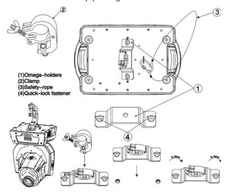
Screw one clamp each via a M12 screw and nut onto the Omega holders. Insert the quick-lock fasteners of the first Omega holder into the respective holes on the bottom of the Vizi Beam 5R. Tighten the quick-lock fasteners fully clockwise. Install the second Omega holder. Pull the safety-cable through the holes on the bottom of the base and over the trussing system or a safe fixation spot. Insert the end in the carabine and tighten the safety screw.
