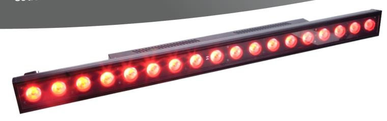
The ADJ Mega TRI Bar 1.1-meter indoor LED Bar features 18 TRI Color LEDs of 3W rated at 60,000 hours with built-in Pixel Control and a wide beam angle of 40 degrees. It can run in stand-alone mode with its built-in programs or be controlled by DMX via 7 different DMX Modes. It has locking 3-pin DMX and IEC In/Out connections to daisy-chain data & power.
