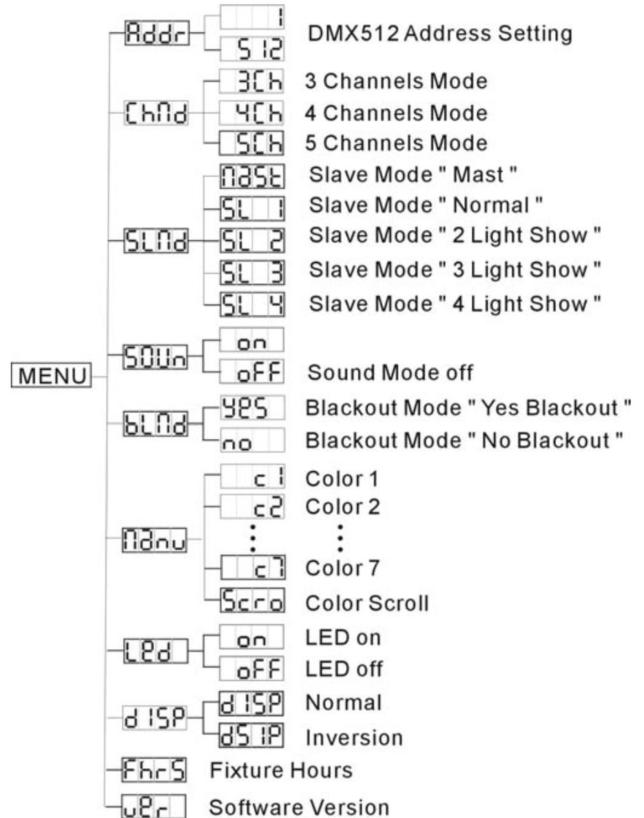
**System Menu:** When making adjustments you can press **ENTER** to confirm your setup or you can wait 8 seconds for automatic setup. To exit without making any adjustments press the **MENU** button.
