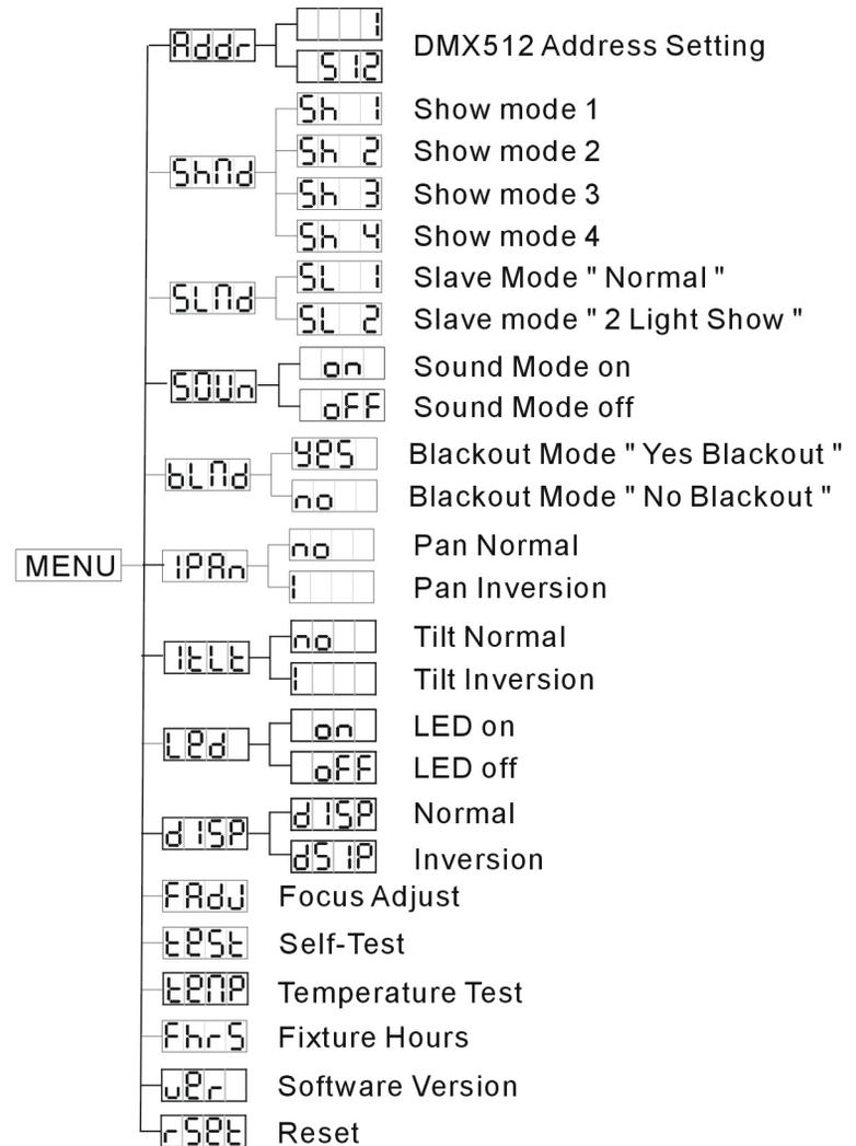
**System Menu:** When making adjustments you can press **ENTER** to confirm your setup or you can wait 8 seconds for automatic setup. To exit without making any adjustments press the **MENU** button.
