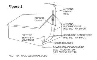
Article 810 of the National Electrical Code, ANSI/NFPA 70, provides information with regard to proper grounding of the mast and supporting structure, grounding of the lead-in wire to an antenna discharge unit, size of grounding conductors, location of antenna-discharge unit, connection to grounding electrodes, and requirements for the grounding electrode.
