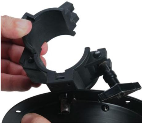
Attach the clamps securely to the mounting holes on the motor. Make sure the clamps are firmly attached to the motor before mounting to the truss.
