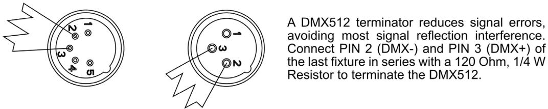
**5-Pin XLR DMX Connectors:** Some manufacturers use 5-pin DMX-512 data cables for DATA transmission in place of 3-pin. 5-pin DMX fixtures may be integrated into a 3-pin DMX line with a 5-pin to 3-pin adapter cable. These adapters are readily available at most electronics stores. Follow the chart below for a proper conversion.
