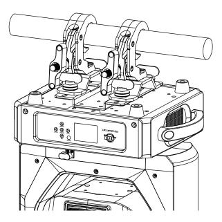
When mounting fixture to truss, be sure to secure an appropriately rated professional grade rigging clamp to the included **Omega Brackets** using an M10 screw fitted through the center hole of the **Omega Brackets**. The fixture provides built-in rigging points for a **SAFETY CABLE** (not included). Be sure to only use one of the designated rigging points for the safety cable and never secure a safety cable to a carrying handle.
