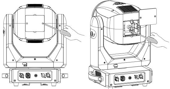
Lift lamp out of its recess and replace it with an OSRAM SIRIUS HRI® 310W PRO lamp. Reassemble in reverse order.
