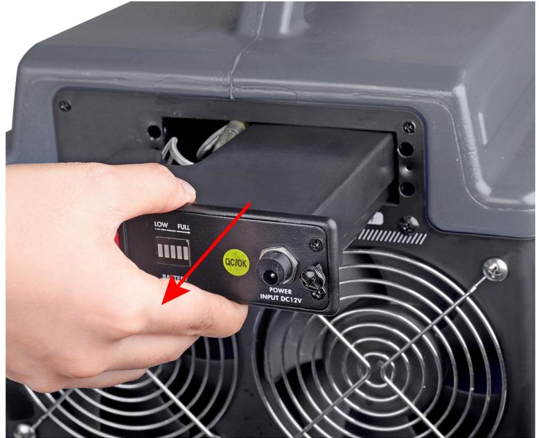
2. Locate and disconnect the wire connector on the back side of the battery pack. Fully remove the old battery from its slot, and install a replacement by reversing these steps.
