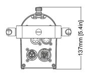
Note: Height may depend on thumb screw tightness. Overall height when fully tightened is 137mm (5.4in) as shown below. Overall height with thumb screw loosened is 140mm (5.5in).
