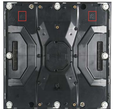
Pull the LED module away from the video panel frame, as shown in the above left image. Grasp the freed LED module securely with your free hand, then press and release the trigger on the vacuum tool to disengage suction. When re-assembling, ensure that the arrow on the frame (above center) is aligned in the same direction as the arrows on the back of the LED module (above right).
