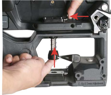
2. Press spring-loaded locking latch to the left while pressing vertical connector upwards into locking latch.
