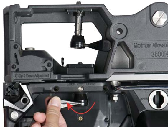
3. Release latch to hold the vertical connector, and twist vertical connector the left to lock.
