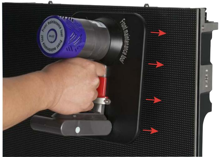
Detach the safety cable for the LED module that you wish to remove. The above left image, for example, shows the location of the safety cable for the upper left LED module. Next, gently press the cushioned face of the vacuum tool to the front of the LED module, as shown in the above right image, and press and release the trigger. Please note that you do not need to continuously hold the trigger to maintain suction.
