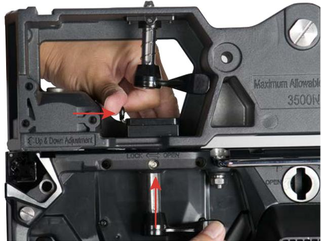
2. Press spring-loaded locking latch to the right while pressing vertical connector up into locking latch.
