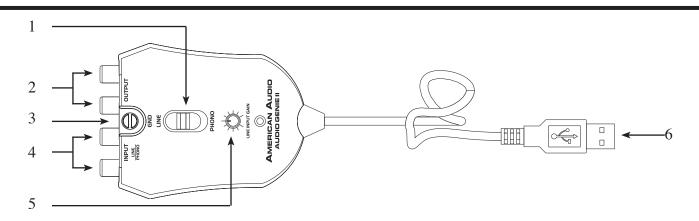
**1.** *Line In/Phono Switch -* This switch is used to select the input source assigned to the input jacks. The button must be in the "Phono" position for turntable operation.
