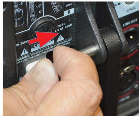
Pull **Linkpin 2** from integrated adjustable mounting bracket of the top **IMPERIO** speaker.
