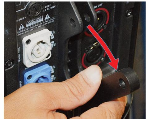
Swing integrated adjustable mounting bracket down.
