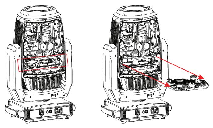
4. Pull the gobo holder away from the gobo wheel, then gently slide it outwards. Use a pair of needle nose pliers to carefully remove the retainer spring from the gobo holder. The gobo can now be removed from the gobo holder, and replaced with a new gobo. Reassemble by reversing these steps.
