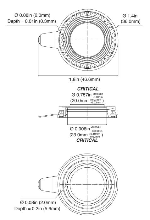
Note: Dotting and milling slot on the same tooth tip.
