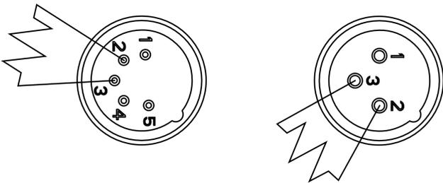
A DMX512 terminator reduces signal errors, avoiding most signal reflection interference. Connect PIN 2 (DMX-) and PIN 3 (DMX+) of the last fixture in series with a 120 Ohm, 1/4 W Resistor to terminate the DMX512.
