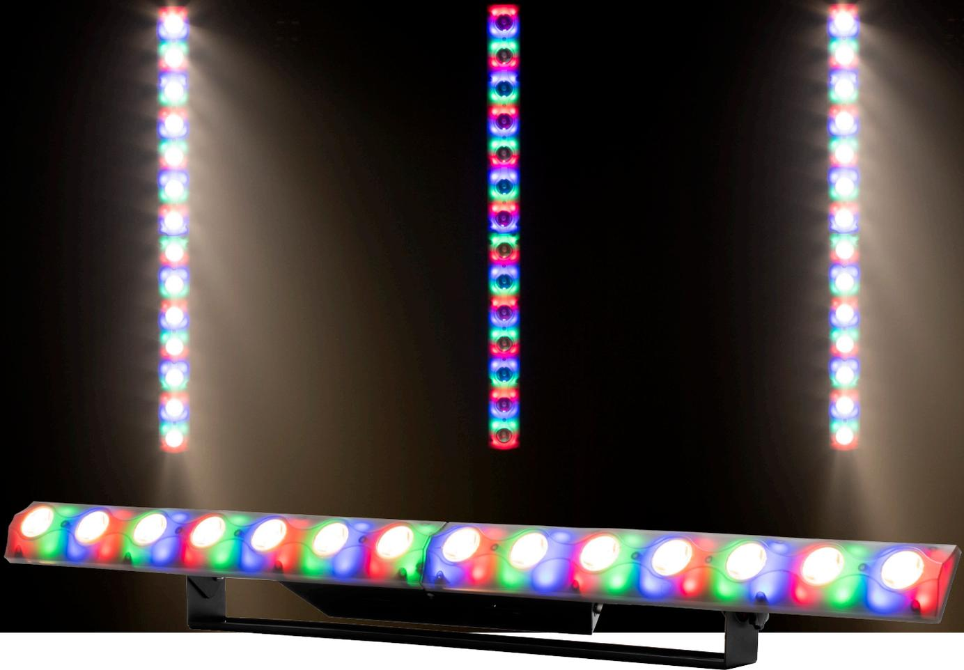
The **Eliminator Lighting Frost FX BAR W** is a 1-meter linear entertainment lighting fixture that creates color washes and breathtaking color chase effect. It has two types of color LEDs in one fixture. It has fourteen 3W white LEDs with ACL lens across the front of the fixture to create intense beam effects. Plus, it has eighty-four RGB SMD LEDs behind a frosted plastic lens that create glowing color chase patterns. Both sets of LEDs run independently.
