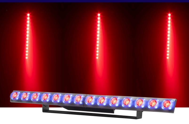
The **Eliminator Lighting Frost FX BAR RGBW** is a 1-meter linear entertainment lighting fixture that creates color washes and breathtaking color chase effect. It has two types of color LEDs in one fixture. It has fourteen 3W RGBW LEDs with ACL lens across the front of the fixture to create color beam effect. Plus, it has eighty-four RGB SMD LEDs behind a frosted plastic lens that create glowing color chase patterns. Both sets of LEDs run independently.
