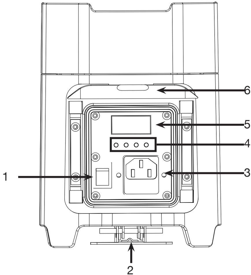
1. **Battery On/Off Switch:** This switch is used to turn ON battery power and also turn ON the PCB output. See page 17 “**Load Setting**” to activate.
