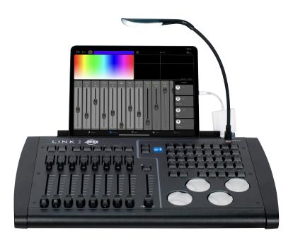
LINK is a 4-universe controller designed to control compatible DMX devices with control from the dedicated Airstream LINK iOS App for iPad.
