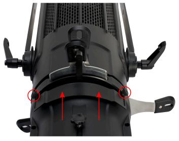
4. Slide the plate back to cover the iris slot, and tighten the thumb screws to secure in place. The plate should be in contact with the handle of the iris, but be careful not to push the plate too tightly against the handle. Do not overtighten the thumb screws.
