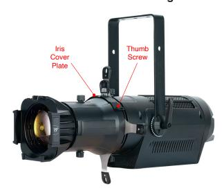
Locate the iris cover plate at the top of the fixture, just forward of the blade shutters. Loosen (but do not completely remove) the two thumb screws that hold the plate in place, then slide the cover plate forward to expose the iris slot.
