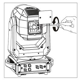
Carefully lift the lamp out of its recess, disconnect the lamp, and replace it with a new Philips MSD Platinum 12 R LL lamp.
