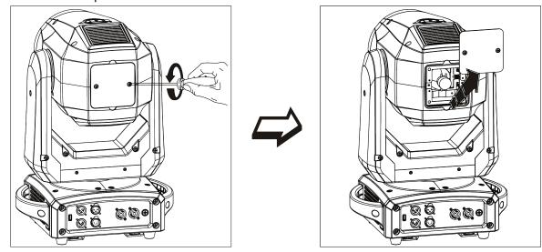
Loosen the two screws in the recess.
