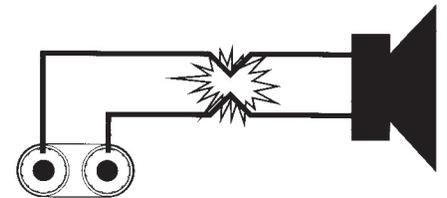
put). *Short Circuit Protection* can usually be traced back to the signal output line (i.e. speaker line). Check the line from the output terminal of the amplifier to the speaker. If this line good, check the internal speaker connections and components. A short circuit will usually be traced to a bad cable or a bad speaker component and is rarely traced to the amplifier itself.
