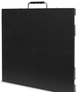
The AV4XIP is a high resolution video panel from ADJ. Each panel has a pixel pitch of 4.81mm with a configuration of a 3-in-1 RGB SMD1921 LED's. The panel is IP65 on the front and IP54 on the back, which allows for temporary outdoor use. The brightness is 4000 NITS. There are 2 LED modules per panel. This allows for easy serviceability. The AV4IP includes IP65 locking power in/out connections and locking RJ45 ethernet in/out connections. This panel also features a Novastar receiving card.
