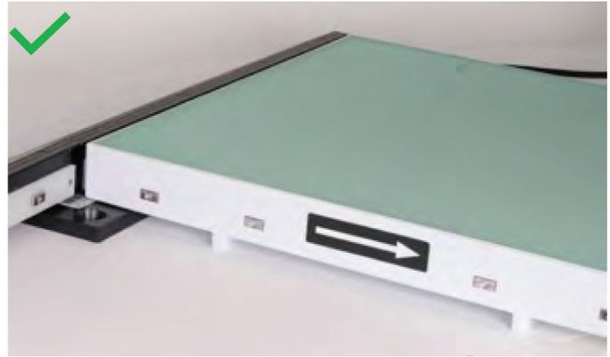
5. Connect a panel to any of the power supply ramps using the docking magnets, making sure that each foot on the panel slots into the holes in the Connection Brackets. Adjust the position of the Connection Brackets as needed to align them with the panel feet. The panel itself should be oriented so that the arrows on each side of the panel are pointing directly away from the power supply ramp.
