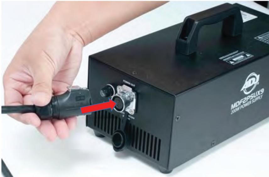
3. Connect your row of Panel Power Ramps to both the DMX console and the Power Supply. Plug in the Power Supply and switch it on.
