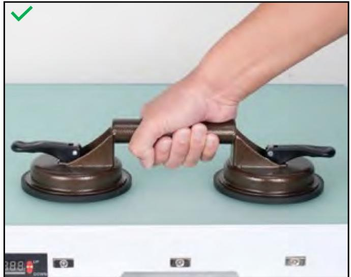
2. Use the Grip Handle to press the Suction Cup Discs firmly against the lighting surface of the Magnetic Dance Floor Panel and move both Suction Cup Levers to the downward position. The Panel Removal Tool should now be firmly attached to the Magnetic Dance Floor Panel.
