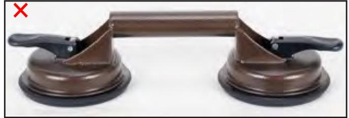
1. Make sure that both Suction Cup Levers are in the upward position.
