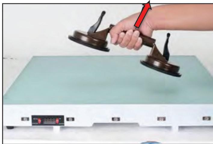
5. The Panel Removal Tool can now be removed from the Magnetic Dance Floor Panel.
