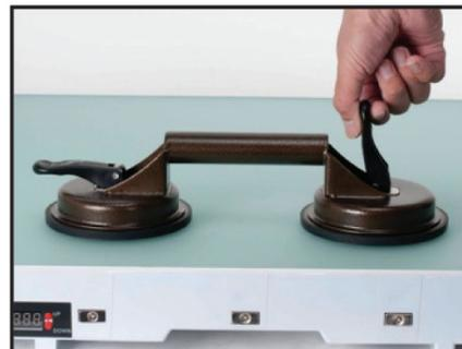
4. To detach the Panel Removal Tool from the Magnetic Dance Floor Panel, move both suction cup levers to the upward position.
