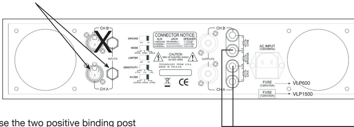
Use the two positive binding post terminals (red) for speaker output.
