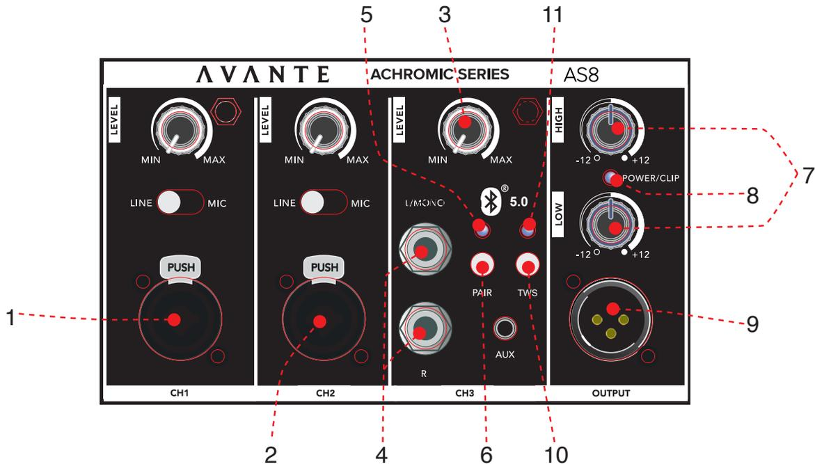
1. **CHANNEL 1:** This input accepts balanced XLR plugs, and balanced/unbalanced TRS (tip/ring/sleeve) 1/4" plugs. Set the LINE/MIC switch to match the type of device that will be connected in order to prevent distortion. When using an unbalanced 1/4" instrument jack, start with the button in LINE setting. Then, if the gain is too low, turn the volume down, select MIC, and slowly raise the volume.
