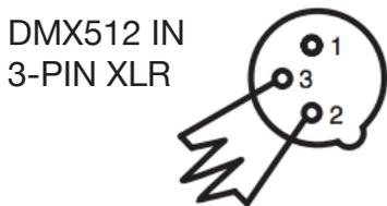
Termination reduces signal errors and avoids signal transmission problems and interference. It is always advisable to connect a DMX terminal, (Resistance 120 Ohm 1/4 W) between PIN 2 (DMX-) and PIN 3 (DMX +) of the last fixture.
