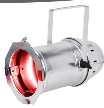
The Par ZP120 RGBW is a modern LED twist to the traditional halogen Polished Par Can. It is powered by a potent 115W quad C.O.B. LED (Chip On Board) LED with red, green, blue & white colors. Its output is comparable to a 1000W halogen sealed beam Par. It is equipped with 5 different beam angle options that may be changed by hand. Locking Power In/Out allows for the fixture to be daisy chained, while 5-pin DMX control offers a variable strobe rate and 5 different dimming curve options.
