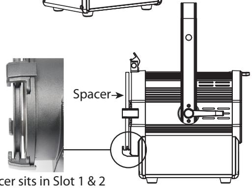
2. Slide the Barn Door in from the top, in front of the Spacer. The Barn Door will sit in the 1st slot.
