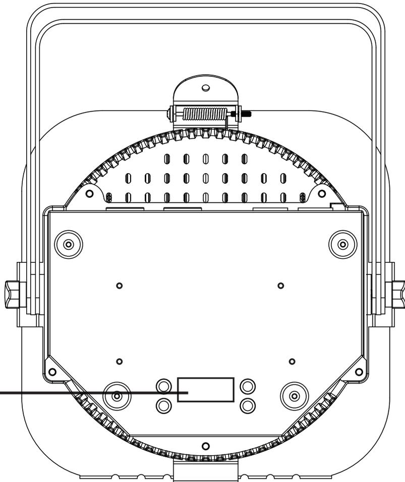
**DMX-512:** DMX is short for Digital Multiplex. This is a universal protocol used as a form of communication between intelligent fixtures and controllers. A DMX controller sends DMX data instructions from the controller to the fixture. DMX data is sent as serial data that travels from fixture to fixture via the DATA “IN” and DATA “OUT” XLR terminals located on all DMX fixtures (most controllers only have a DATA “OUT” terminal).
