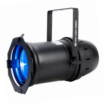
The Par Z120 RGBW is a modern LED twist to the traditional halogen Par Can. It is powered by a potent 115W quad C.O.B. LED (Chip On Board) LED with red, green, blue & white colors. Its output is comparable to a 1000W halogen sealed beam Par. It is equipped with 5 different beam angle options that may be changed by hand. Locking Power In/Out allows for the fixture to be daisy chained, while 5-pin DMX control offers a variable strobe rate and 5 different dimming curve options.
