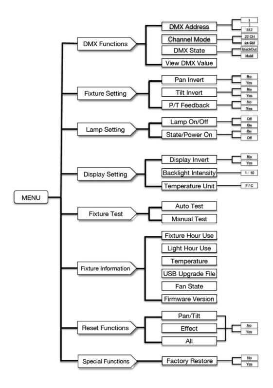
System Menu: When making adjustments press ENTER to confirm your setup then press and hold the MENU button for at least 3 seconds. To exit without making any adjustments press the MENU button. The display will lock after 30 seconds; press the MENU button for 3 seconds to unlock.
