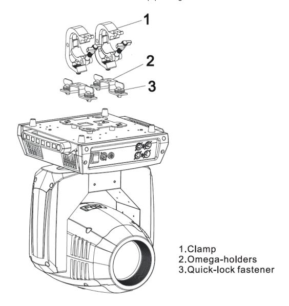
Screw one clamp each via a M12 screw and nut onto the Omega holders. Insert the quick-lock fasteners of the first Omega holder into the respective holes on the bottom of the Vizi CMY 16RX. Tighten the quick-lock fasteners fully clockwise. Install the second Omega holder. Pull the safety cable through the openings located on the base plate and over the trussing system or a safe fixation spot. Insert the end in the carabineer and tighten the safety screw.
