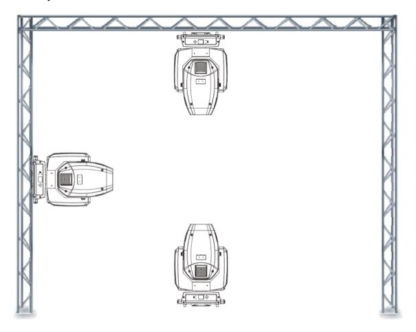
The Vizi CMY 16RX is fully operational in three different mounting positions, hanging upside-down from a ceiling, sideways on trussing, or set on a flat level surface. Be sure this fixture is kept at least 12m (40ft) away from any flammable materials (decoration etc.). Always use and install the supplied safety cable as a safety measure to prevent accidental damage and/or injury in the event the clamp fails (see next page). Never use the carrying handles for secondary attachment.
