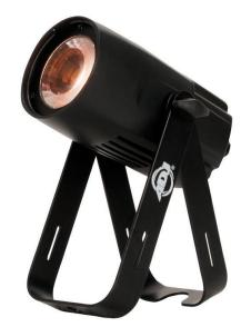
The Saber Spot DTW is a compact spot fixture with a 15-Watt warm white LED. Features DMX-512, flicker-free operation, strobing, electronic dimming and has a 4-Button LED display system on the rear panel. Its built-in ACL lens produces a 20-degree beam angle. It features a dim to warm effect that replicates a halogen-like dimming profile.
