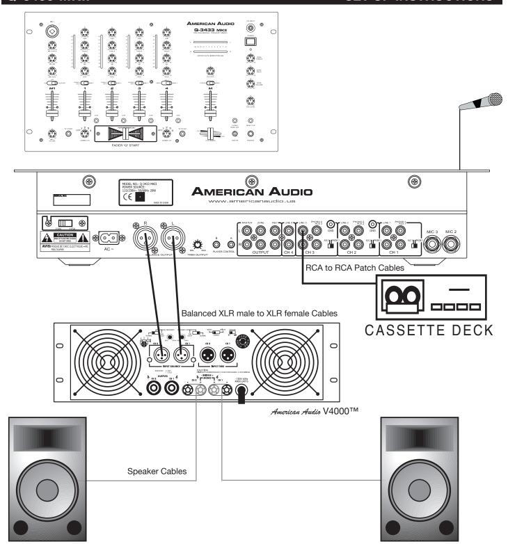
Typical Balanced Output Set-up
